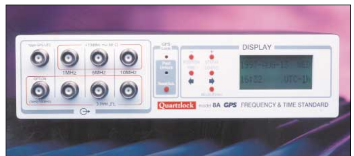
▲ Figure 2. A receiver can recover accurate frequency information transmitted by GPS satellites.
