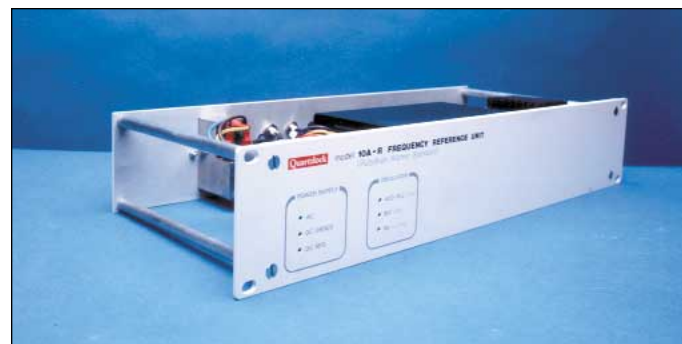
▲ Figure 4. A commercial rubidium standard.
